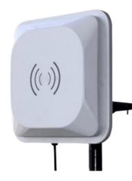
Above: Example of a Static RFID Reader Unit
