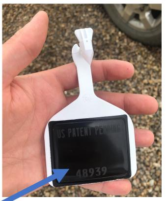
These are the original prototype feedlot tags that were converted to UHF
