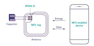
NTAG 22x DNA tags are NFC Forum Type 2 tags and are Common Criteria EAL 3+ certified. There is flexibility to select between two modes to detect tampering: conductive or capacitive tamper detection. There is no need for a dedicated app.
