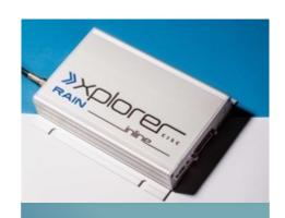
High speed performance testing and encoding of RAIN RFID inlays and tags during production process.
