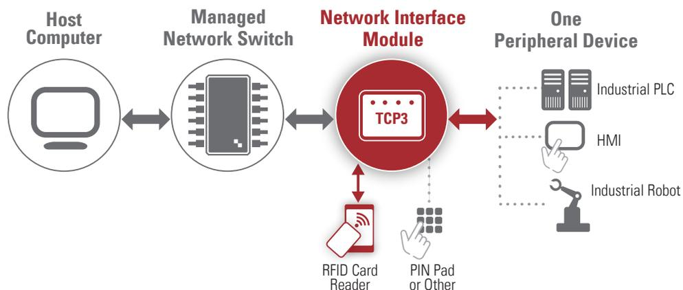
Fig 1. ELATEC Solution – RFID reader + Network Interface Module
