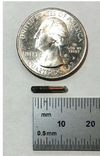
Figure 1. 12mm glass encapsulated FDX RFID tag
