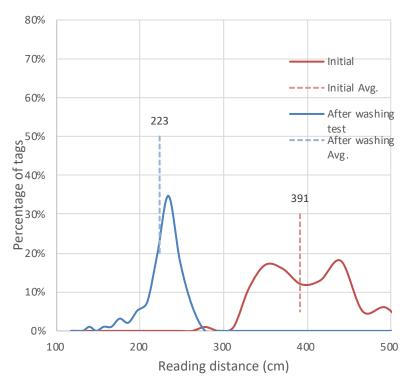
A wide reading range and significant read shift can cause the reading system to lose accuracy over time
