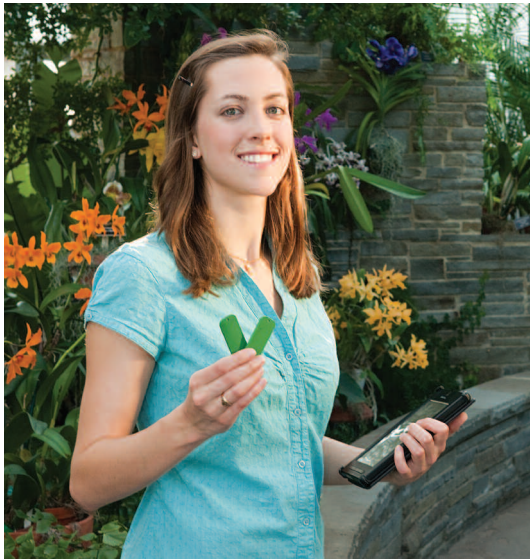
An RFID-enabled Android tablet reads passive UHF tags and automatically plays associated audio clips about the tagged flowers.
