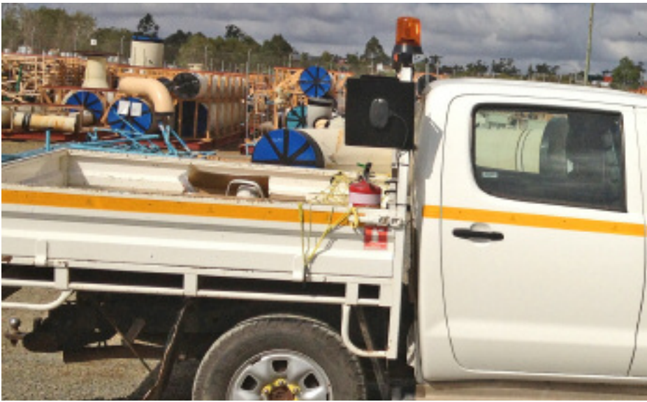
As workers move tagged materials, the new locations are recorded with either vehicle-mounted readers (pictured) or gate readers.
