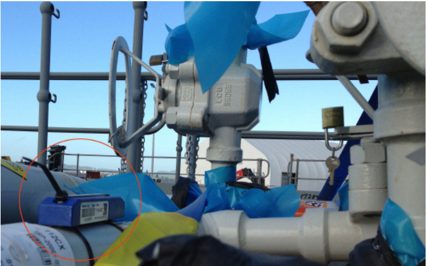
All materials are identified with Identec i-B2 active tags—roughly 60,000 so far. Some tags are recycled, so Bechtel estimates it has tracked well over 100,000 items.
