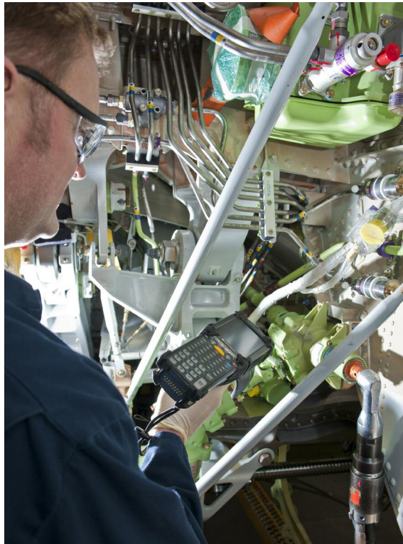
A mechanic reads an RFID tag on a hydraulic motor in a 737 wheel well, during line maintenance.
