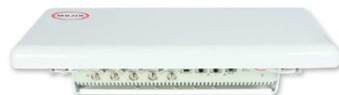
Mojix’s STAR 3000 reader system can identify a passive tag from as far as 600 feet away.
