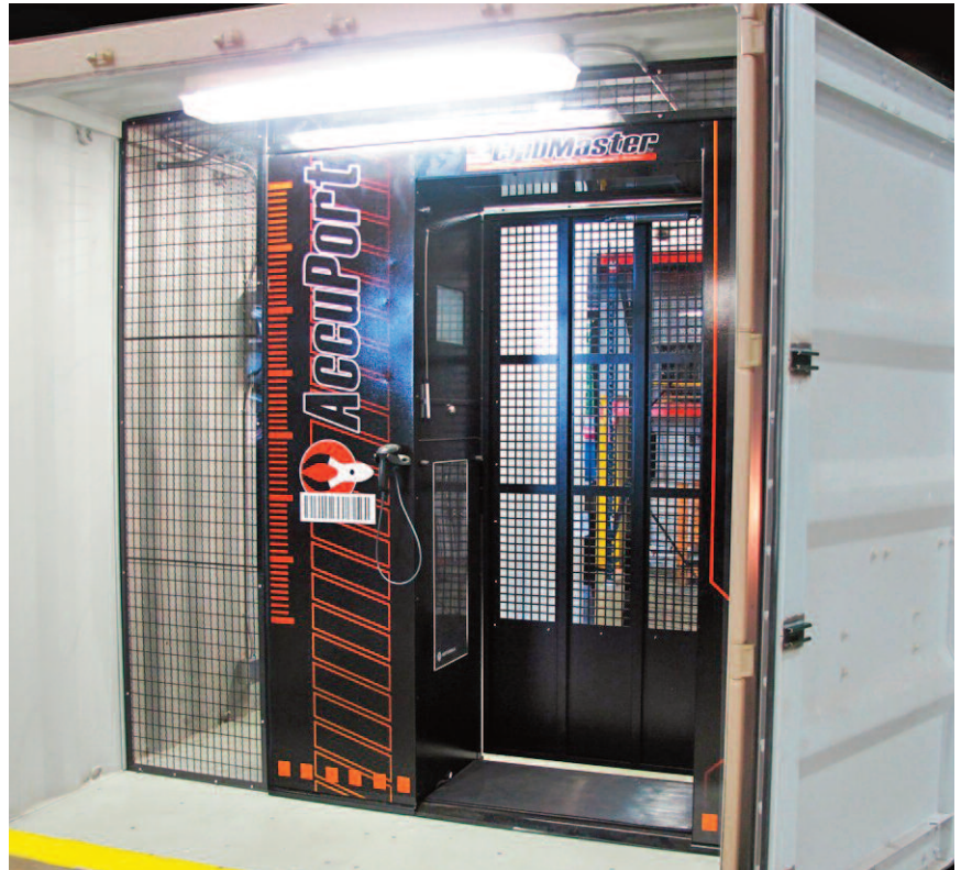
For short-term work, such as jobs at building construction sites, tool-management services generally set up secure, mobile tool cribs.
