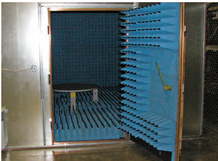
The RFID Research Center's anechoic chamber for testing RFID tags.
