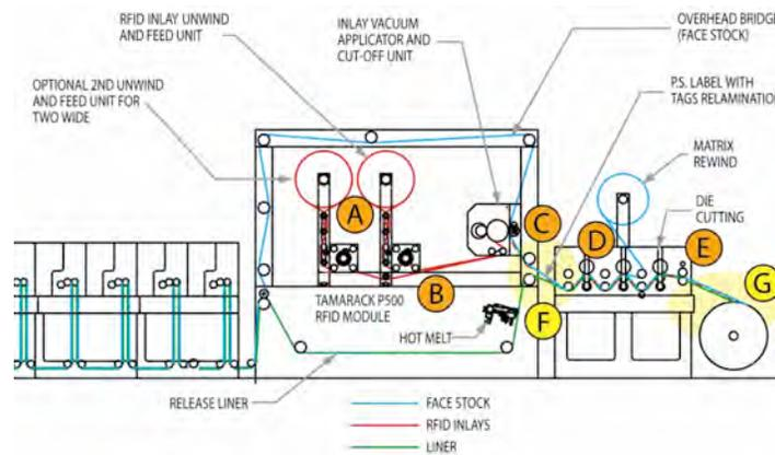
Figure 2 –Areas of possible static generation on an RFID inserter module.
