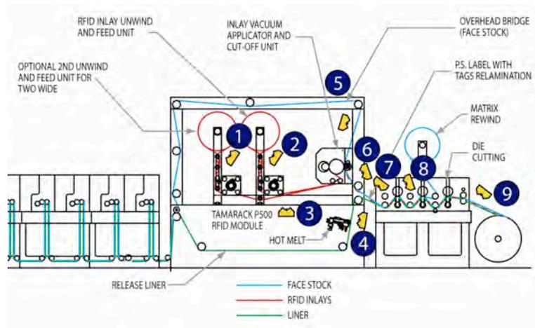
Figure 4 – Recommended locations for static neutralizers in an RFID inserter module.
