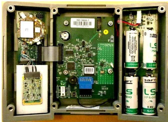
Figure 1. Interior view of an ARG-US RFID tag, with the metal back plate and seal sensor removed. The two devices in the left compartment are the gamma dosimeter (top) and neutron detector.
