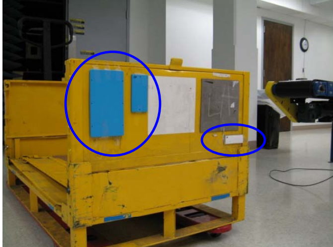
Figure 3: Two hard tags on the left and a label on an RF isolating pad on the right
