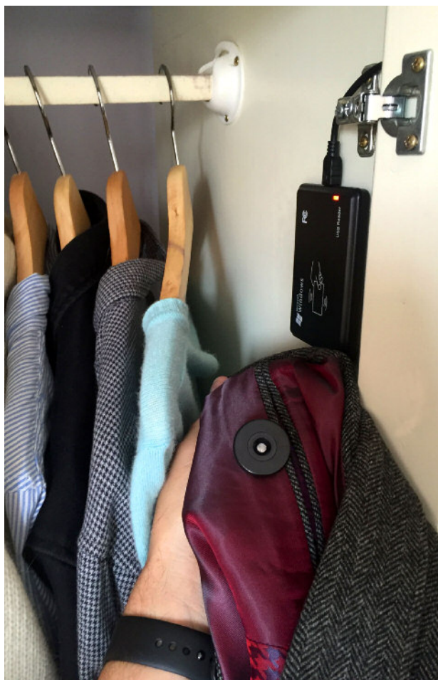
An NFC reader monitors garments identified with NFC laundry tags.
