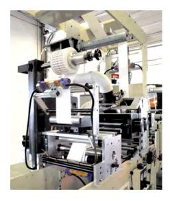
Figure 6 – Placement of static neutralizing bars on an RFID inserter module.
