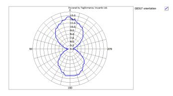
As shown in the illustration above, the orientation pattern of GB3 tag shows that even with the minimum radiation angle at 90 degree and 270 degree, the GB3 tag still achieves a min of 4 meters in theoretical reading distance. (Tested with Voyantic Tagformance system) This omni-directional pattern is very important for retail apparel because the GB3 tag performs in the blind spots that are common in the industry.
