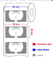
GB3 tag antenna only measures 1.18x1.96 inches which can fit for most of the apparel hang tags or labels. What's more, the GB3 tags can be either converted to hang tags or wet/paperface labels, which can deliver in both single piece or roll format.
