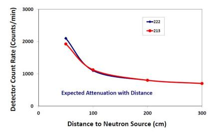
Figure 8. Response of integrated neutron detector tags as a function of distance to the neutron source.
