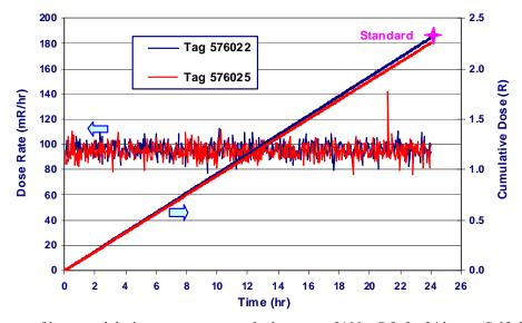
Figure 6. Response of integrated dosimeter tags at a steady dose rate of 100 mR/h for 24 hours (Self-shielding of the front plastic chassis of the tags accounted for the  $\approx 4\%$  reduced readings for both the dose rates and cumulative doses.)
