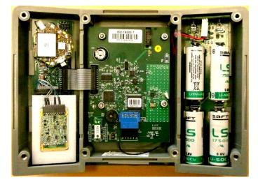
Figure 1. Interior view of an ARG-US RFID tag, with the metal back plate and seal sensor removed. The two devices in the left compartment are the gamma dosimeter (top) and neutron detector.
