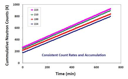
Figure 9. Reliable neutron detector performance as indicated by steady count rates and linear count accumulation over a period of 12 h.
