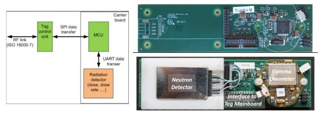
Figure 4. Sketch of interconnections and photos of bare and detector-populated expansion boards.
