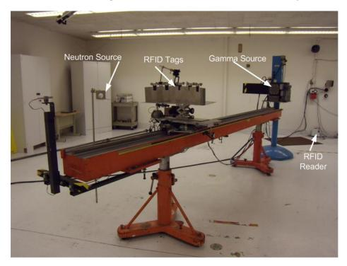
Figure 5. Benchmark testing of integrated-detector tags with a certified Cs-137 gamma source and an AmBe neutron source.
