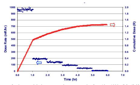
Figure 7. Response of an integrated dosimeter tag at dose rates ranging from 10 to 1000 mR/h. (Self-shielding of the front plastic chassis of the tags accounted for the  $\approx 4\%$  reduced readings for both the dose rates and cumulative doses.)
