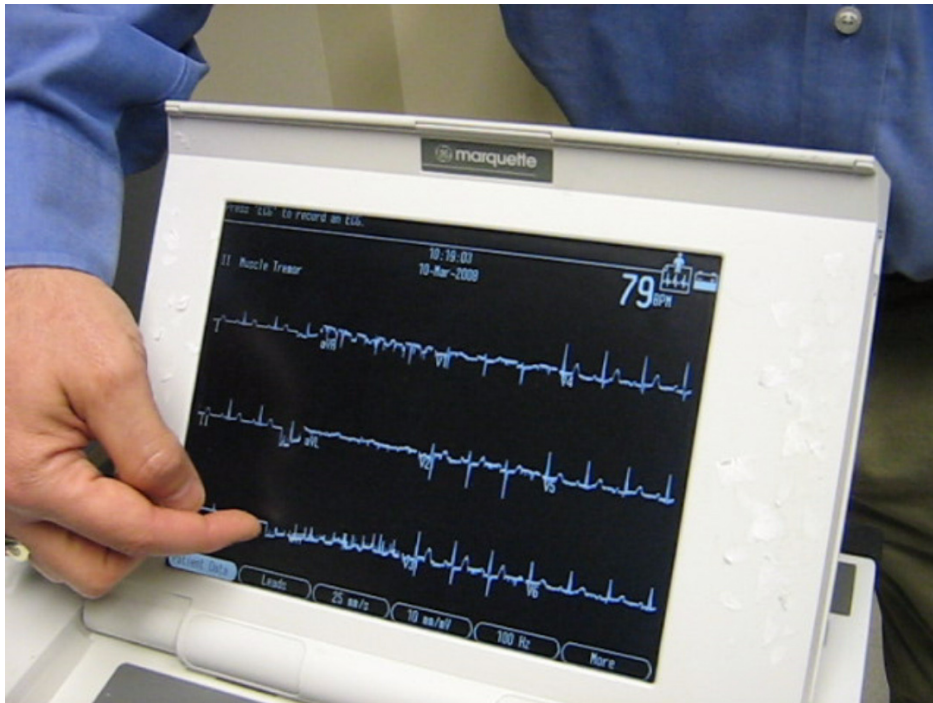
Photo 3 Interference as seen on a 12 Lead EKG recorder
