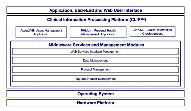
Flexible implementation of CLIP solutions even at the application level is possible due to the innovative modular architecture framework. Modularity allows several elements within CLIP to be added, deleted and/or tested and validated independently. Application interfaces are provided for coupling, decoupling hardware, software, data management and communication layers, back-end applications and services.
