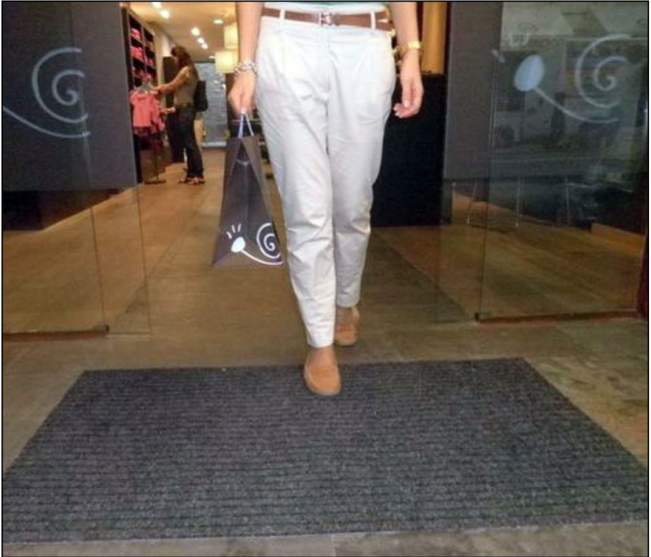
An RFID reader antenna built into a floor mat can be used to determine whether any items leaving the store have not been paid for.
