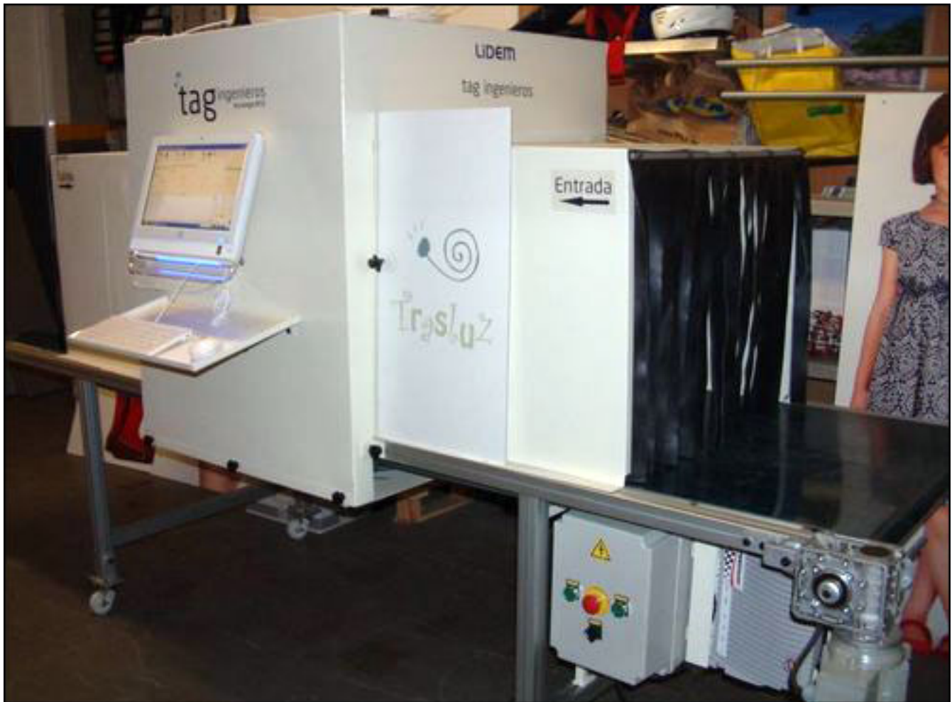
To track incoming and outgoing merchandise at Trasluz's warehouse, workers place boxes of tagged apparel on a conveyor belt with a built-in RFID reader.
