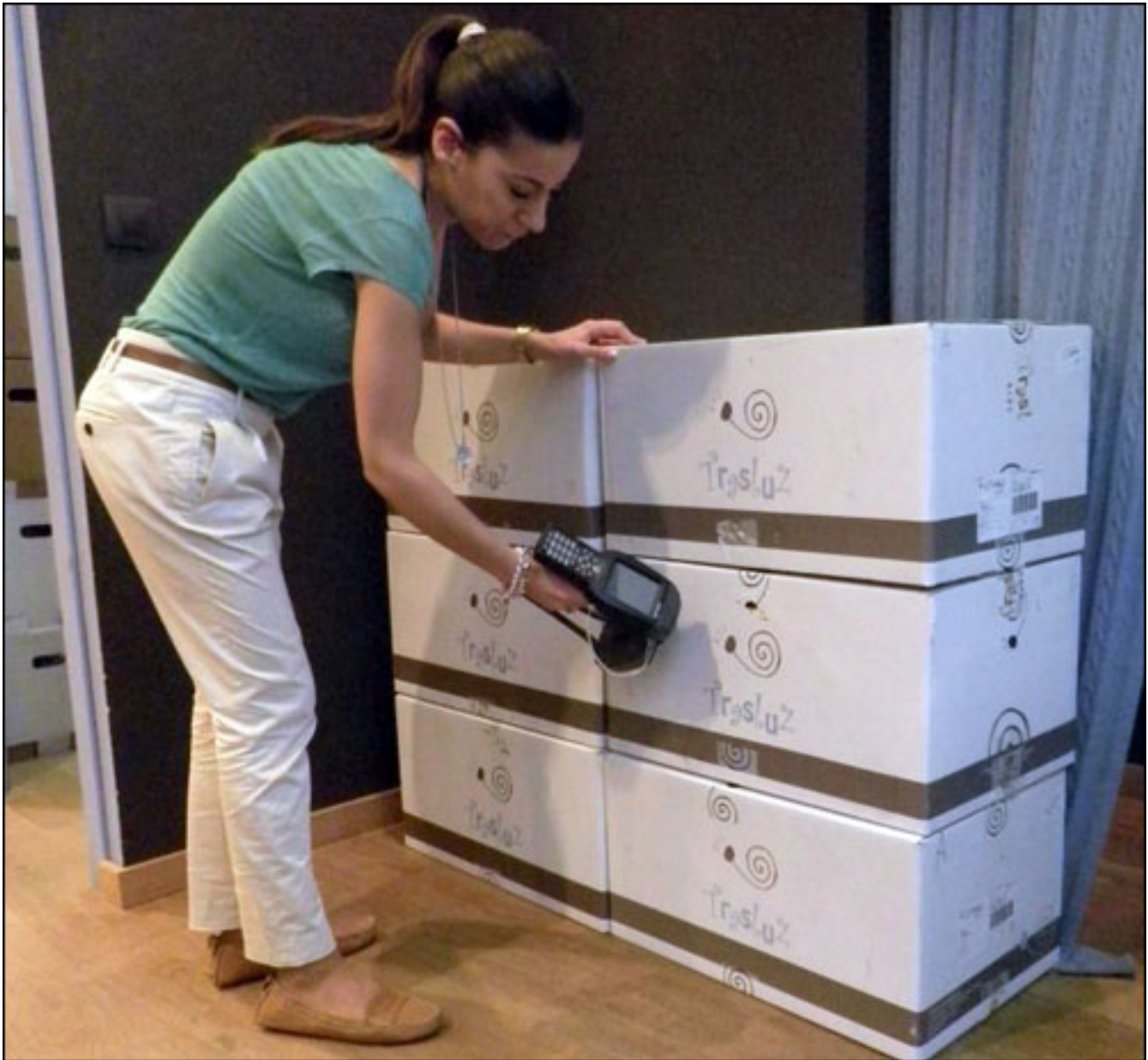
When a shipment of goods is received by a store, workers use a handheld RFID reader to verify the items delivered.
