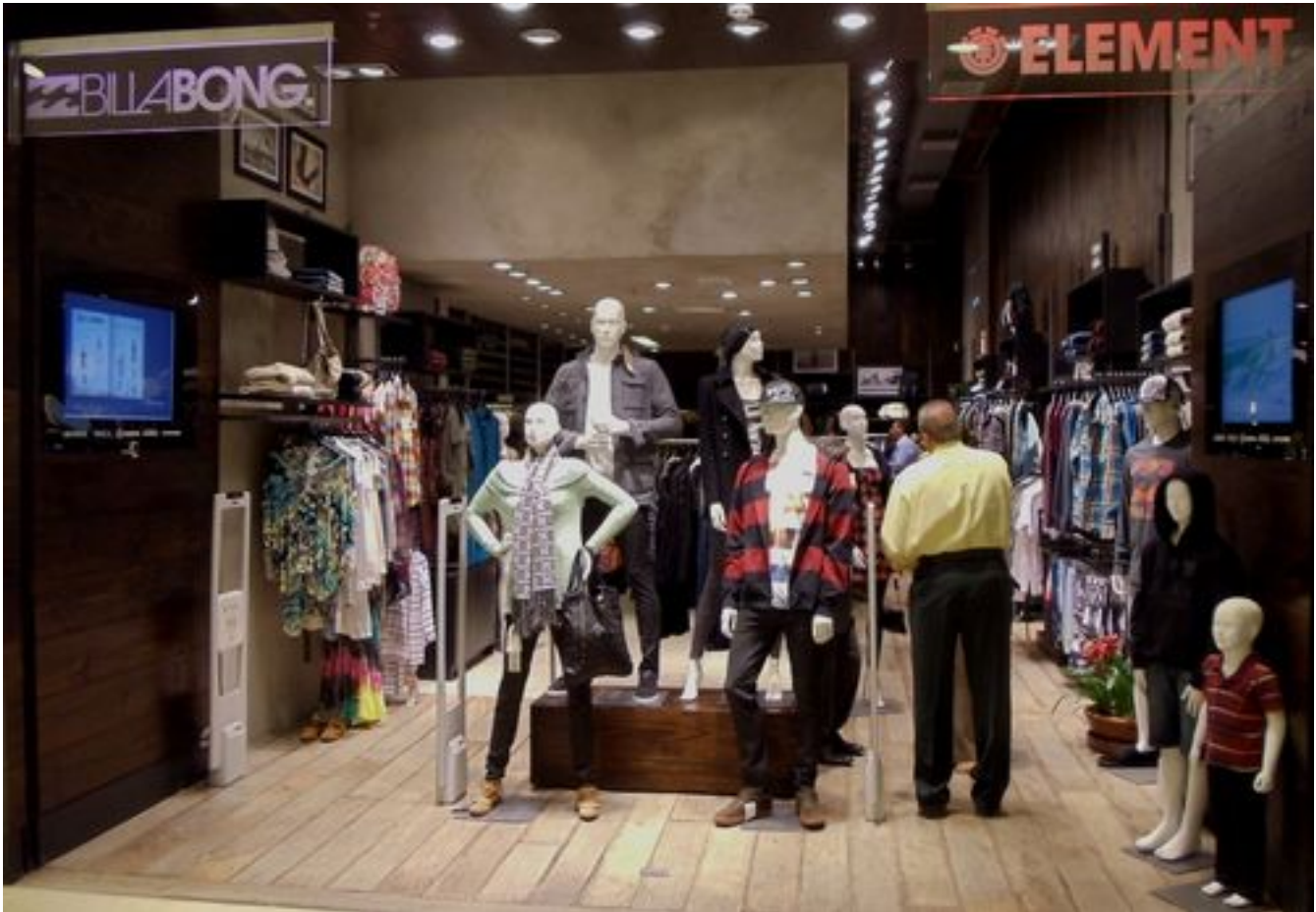
RFID antennas installed at the store's entrance capture the tag ID numbers of merchandise leaving the store, triggering an audible alarm and recording the incident on video if an item was not paid for.
