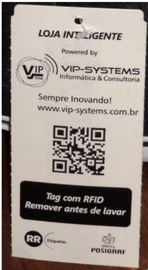
Each piece of merchandise is fitted with a hangtag containing an EPC Gen 2 RFID inlay.
