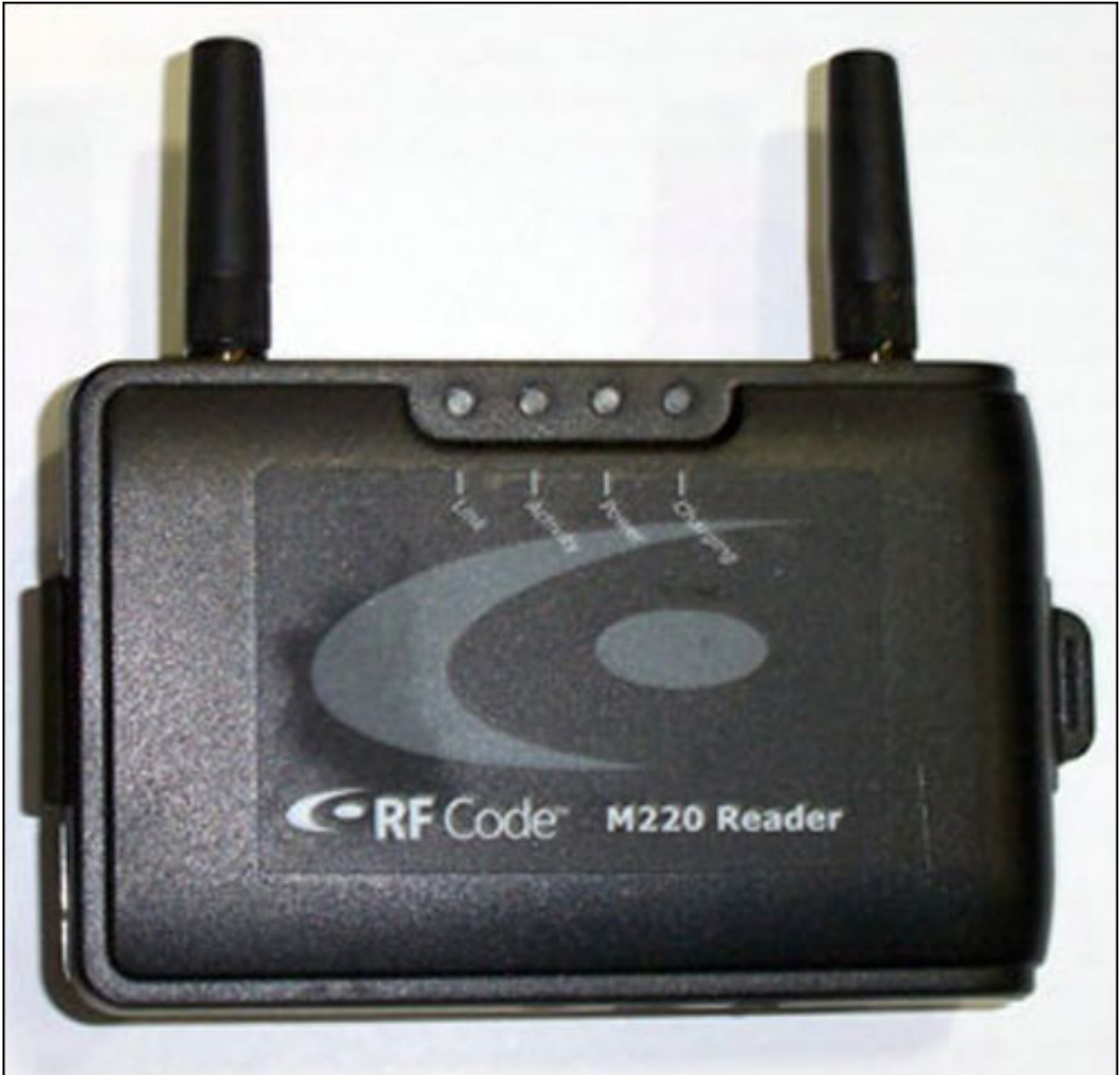
RFID readers are used to identify necessary tools within the warehouse, or to conduct inventory checks.
