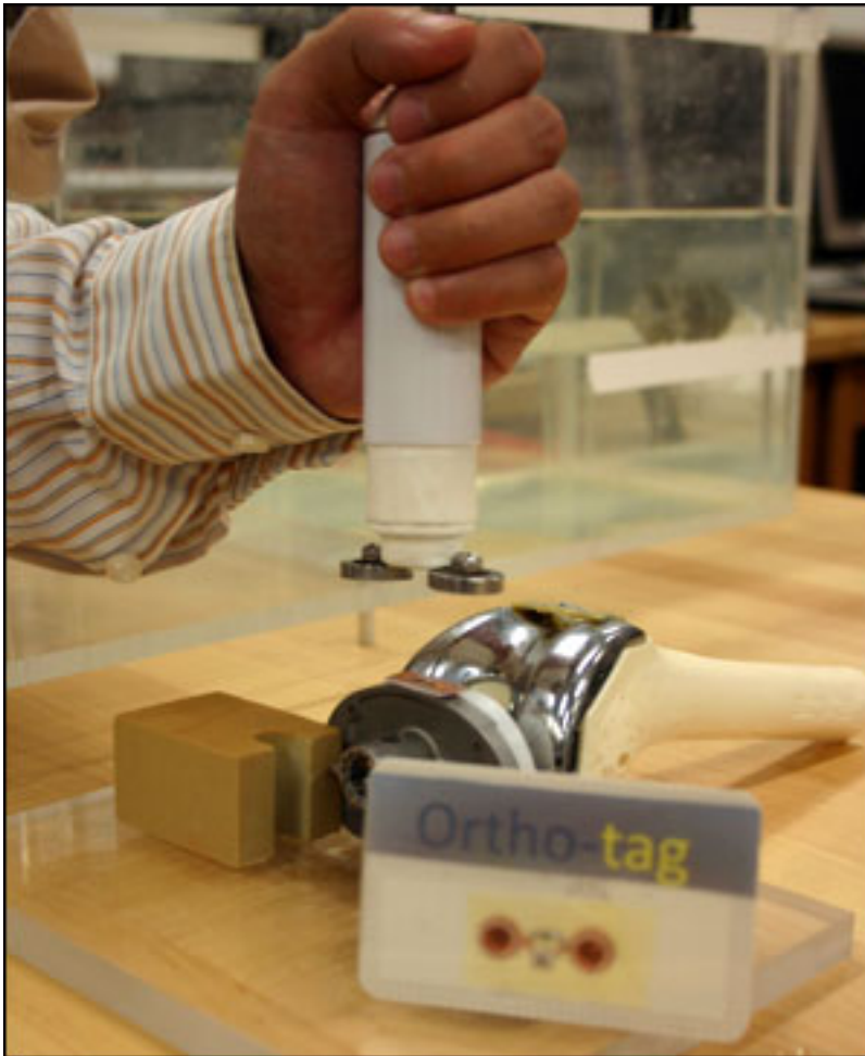
An Ortho-Tag would be affixed to an orthopaedic implant and scanned via an RFID probe. A card (foreground) would be available to patients with an existing implant.
