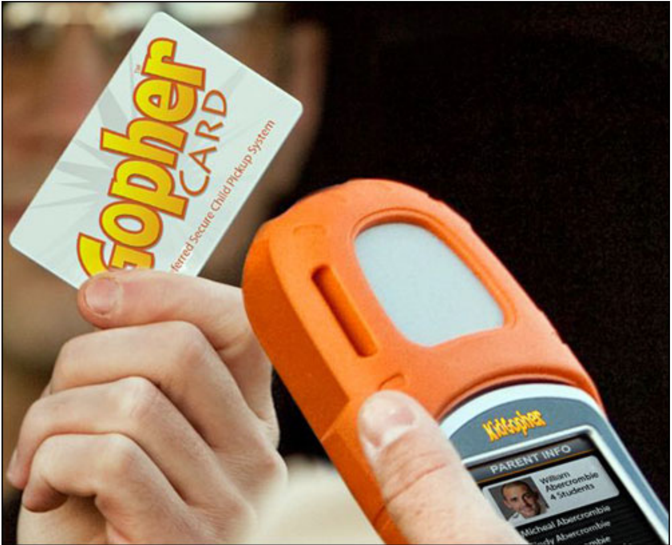
School staff members use a Juniper Systems handheld to read a parent's Gopher card (a SecuraKey card containing a 13.56 MHz RFID inlay).
