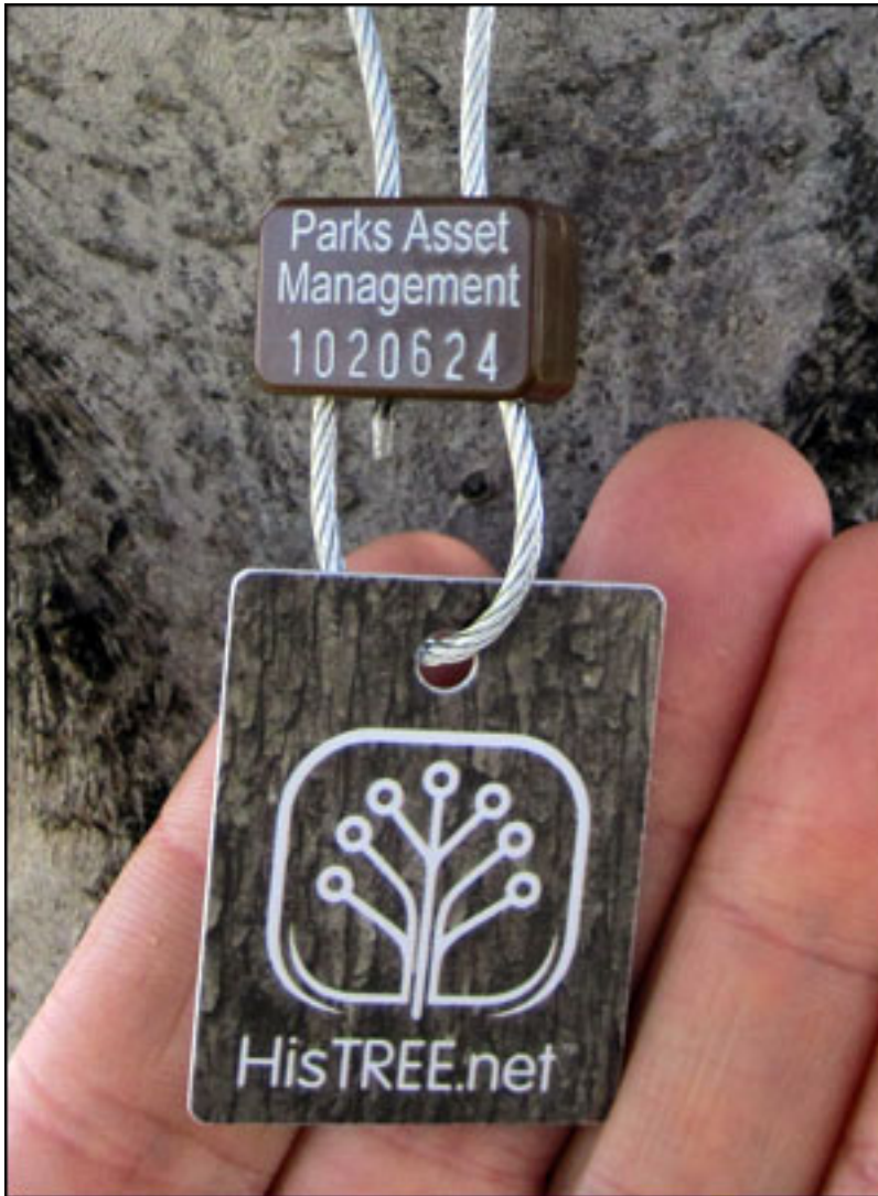
A HisTree.net's tree tag contains a passive EPC RFID inlay.
