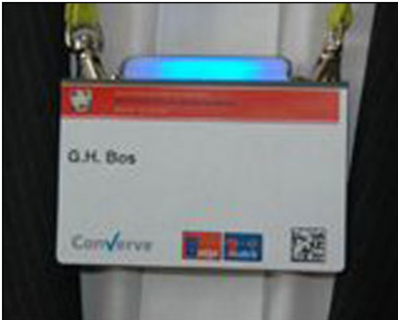
When one person's RFID-enabled SmartBadge detects another badge worn by a person with complementary interests, the two begin flashing the same color.
