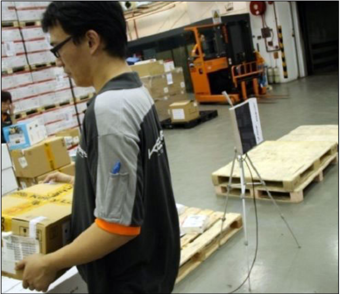
As cartons are loaded onto a pallet, the products' RFID tags are automatically read in order to verify the order is being filled accurately, and to provide a record of what is being shipped.
