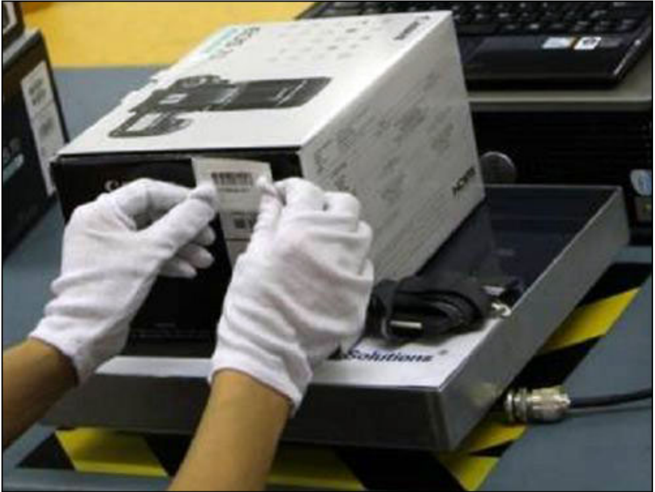
A Kerry Logistics worker applies an Avery Dennison EPC Gen 2 label to the cardboard packaging of each camera or lens.
