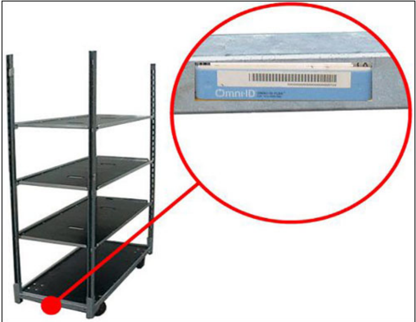
Metal trolleys used for transporting potted plants were fitted with Omni-ID Flex EPC Gen 2 RFID tags.
