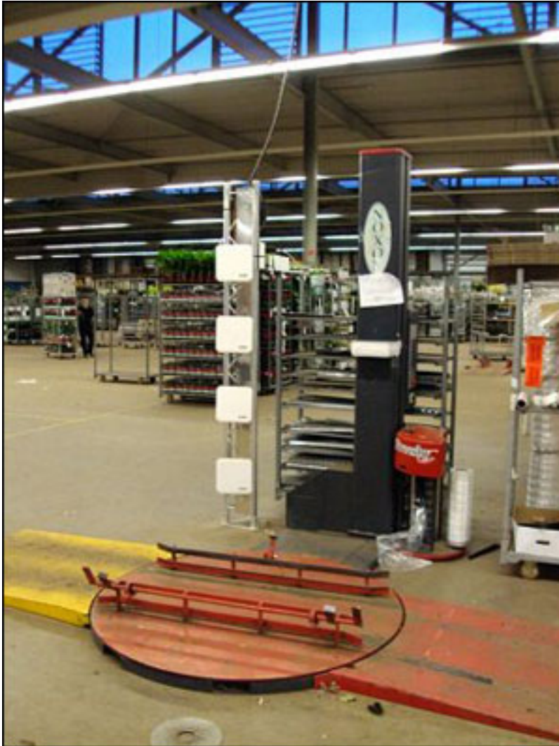
Hamiplant installed an RFID portal where trolleys are repacked with plants to match retailers' specific orders.
