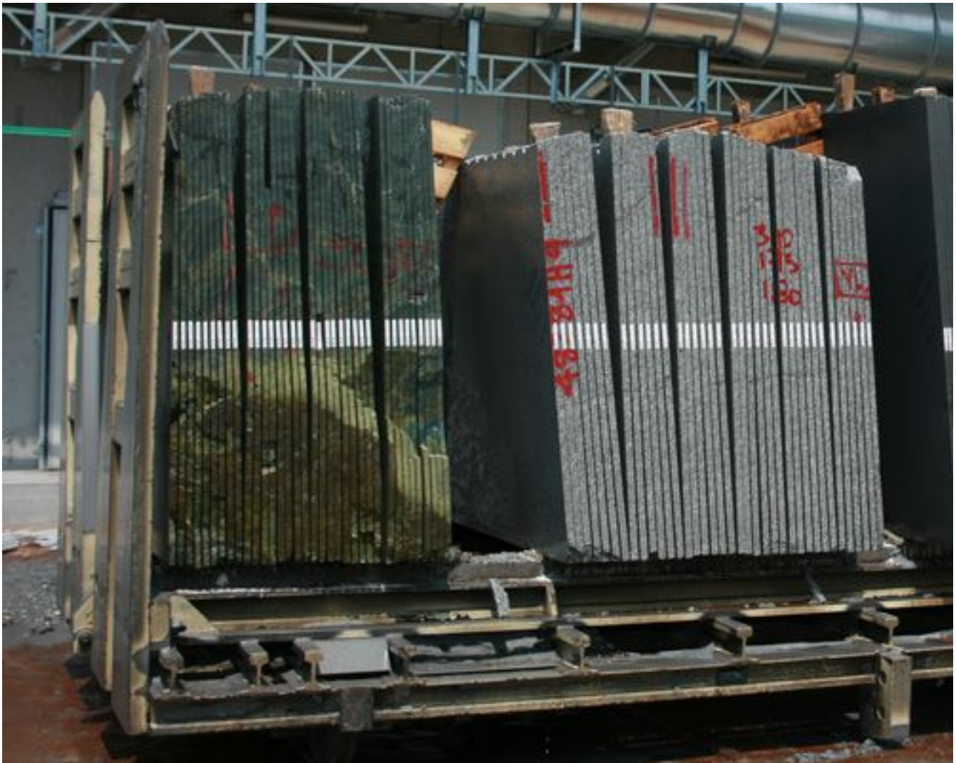
EPC Gen 2 tags embedded in white high-density polyethylene are glued to the edges of finished slabs, which are then stored on racks in the plant's stockyard.
