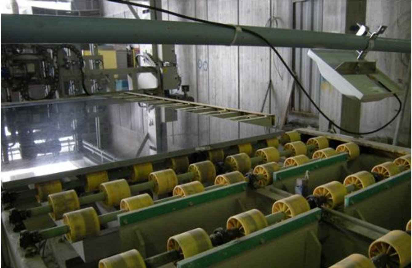
At the company's cutting machine, an RFID antenna is positioned to capture the ID number encoded to a stone block's EPC Gen 2 tag.
