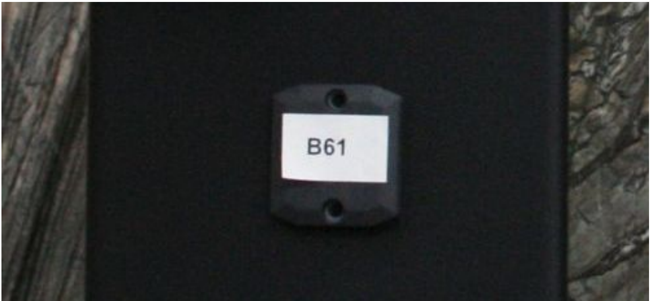
A specialized EPC Gen 2 tag, made by Confidex and designed for mounting onto metal surfaces, is attached to each rack to identify a slab's storage location.
