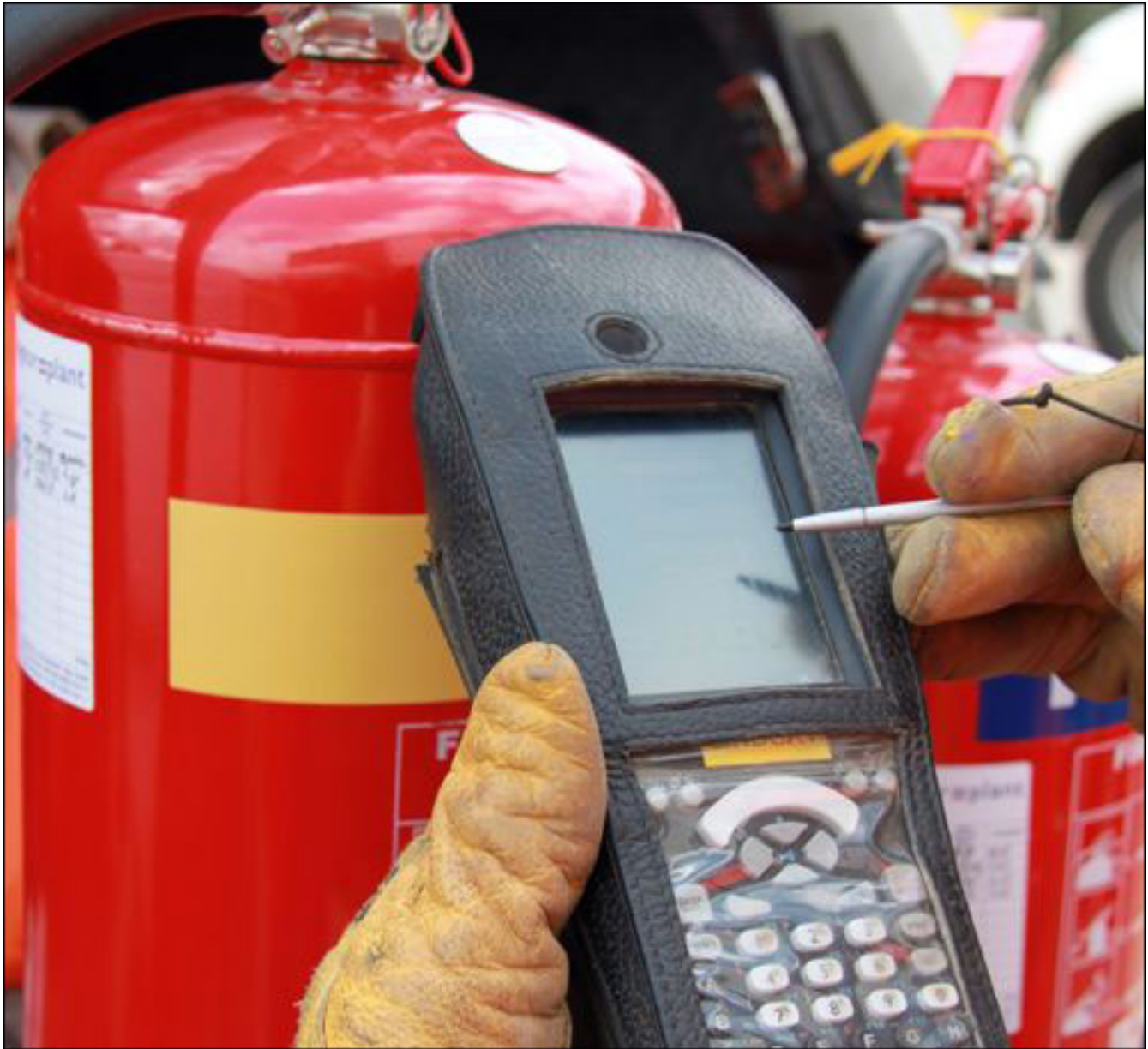
An inspector uses a handheld device to read an RFID tag attached to the top of a fire extinguisher.
