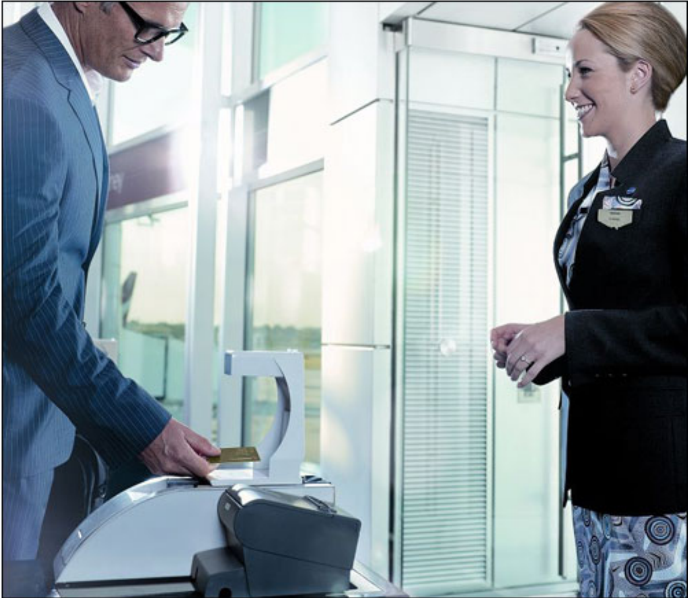
To board a flight, a passenger waves the RFID-enabled frequent-flyer card at the gate to receive a boarding receipt printed with his or her assigned seat number.
