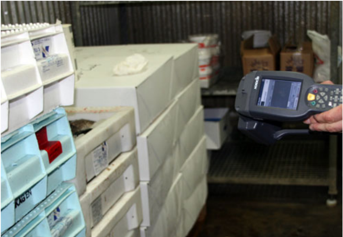
Researchers attached Confidex's Carrier Pro EPC Gen 2 RFID labels to plastic reusable fish containers, and used Nordic ID PL3000 handheld readers to interrogate those tags.
