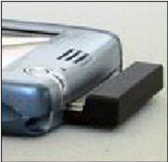
To read the RFID tags attached to chassis and fuel cells, NASCAR's staff uses a Dell Axim x51v PDA with an RFID interrogator.
