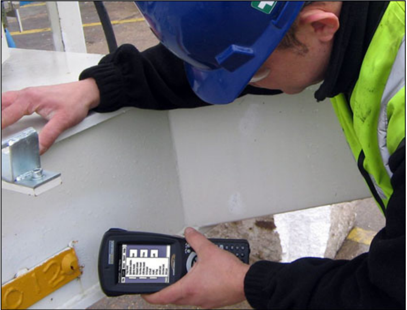
A Byrne employee uses a handheld RFID interrogator to read 125 kHz tag attached to a piece of heavy equipment.
