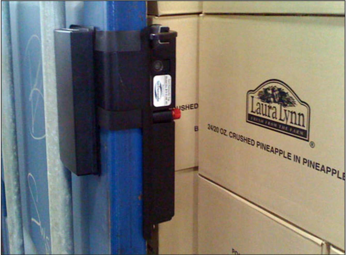
At a food-processing plant in Thailand, workers attached SaviTrak LSE electronic seals to the cargo container doors.
