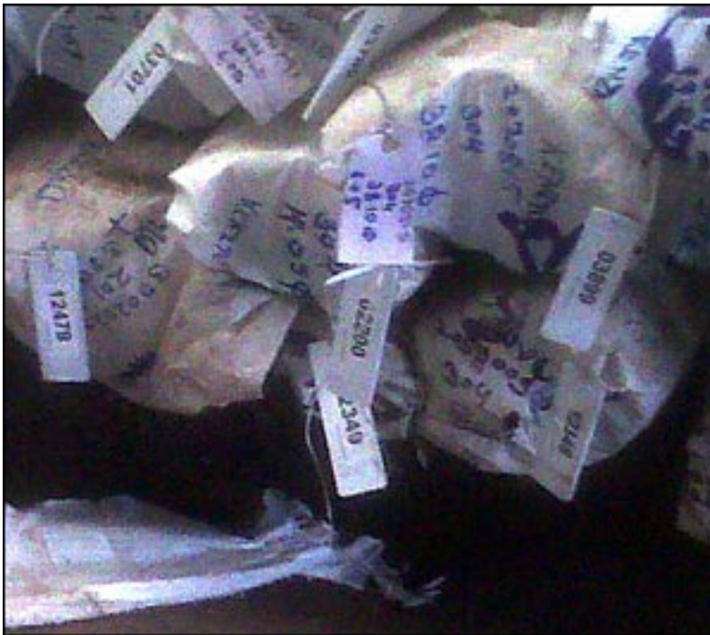
Each bundle is tagged with a UPM Raflatac RFID label with a serial number printed on the surface for visual identification.
