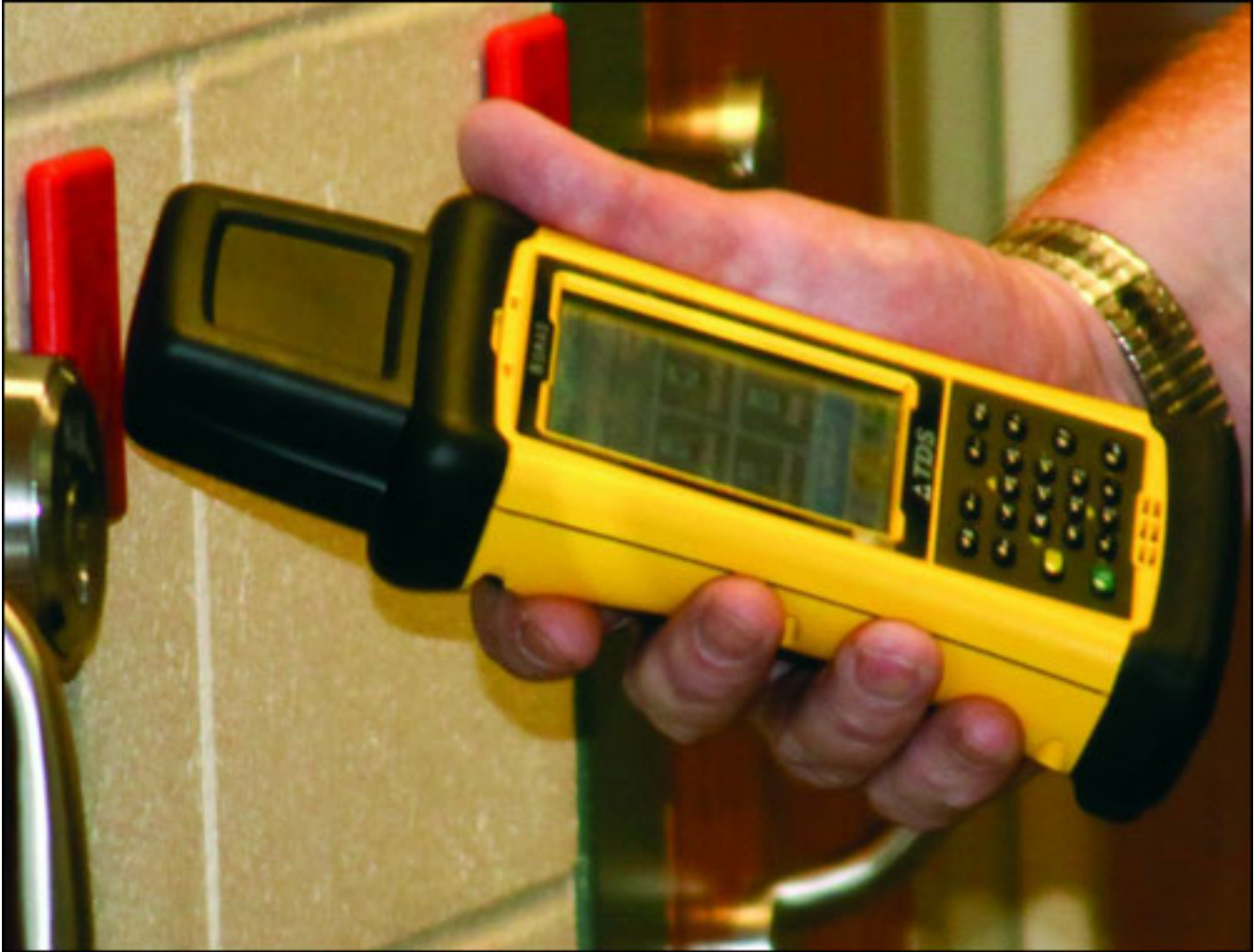
Correction officers use a handheld computer with a CompactFlash RFID reader card to scan the passive RFID tag installed at each cell's doorway.
