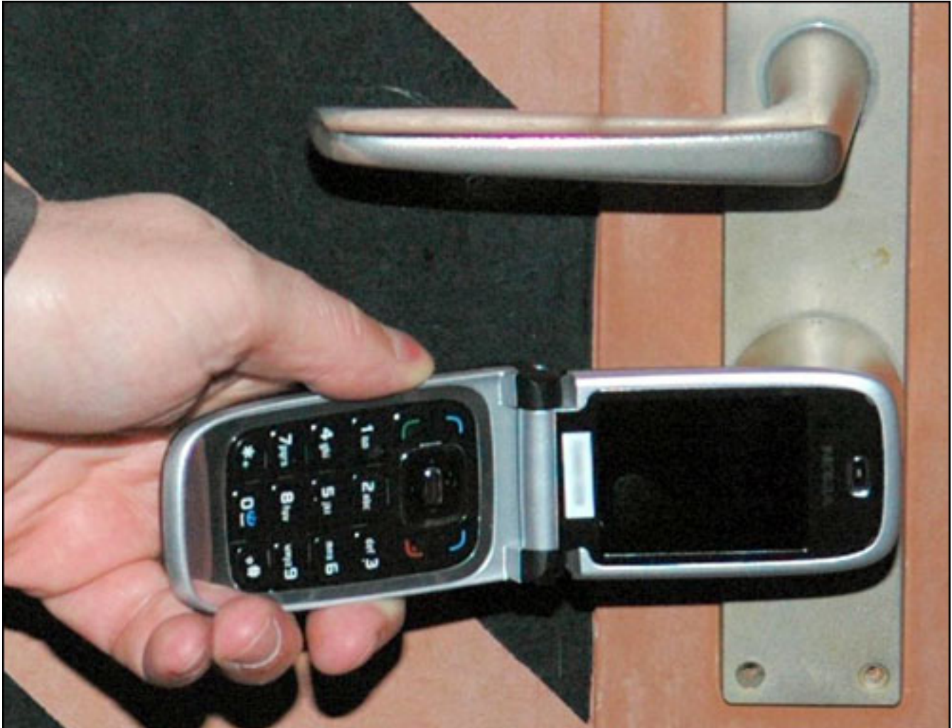
After normal business hours, customers can use the phone's NFC RFID technology to enter the locked store.
