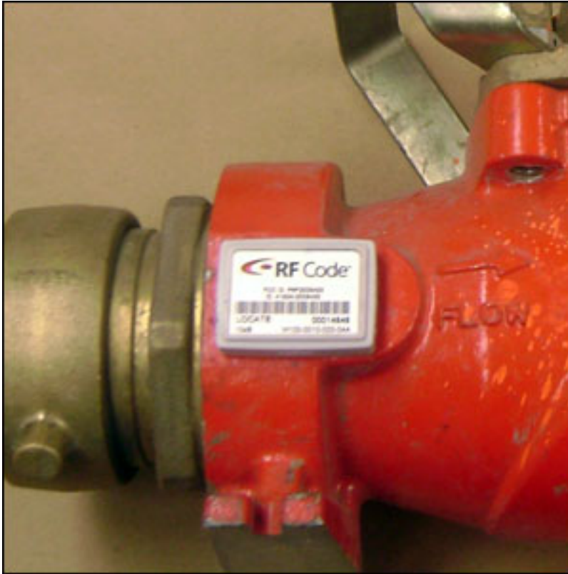
Alco has attached active 433 MHz tags to high-value hardware, such as this construction meter.
