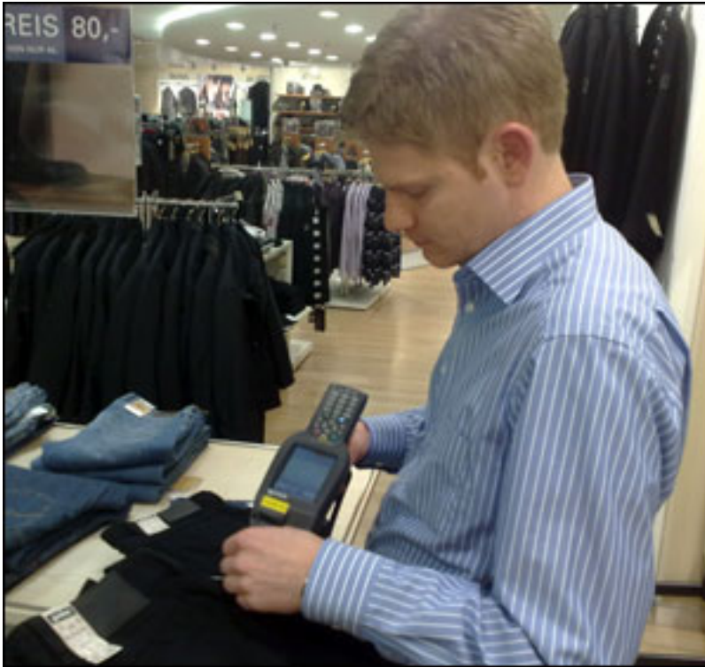
A Jakob Jost employee uses a Nordic ID PL3000 Cross Dipole UHF handheld reader to take inventory.
