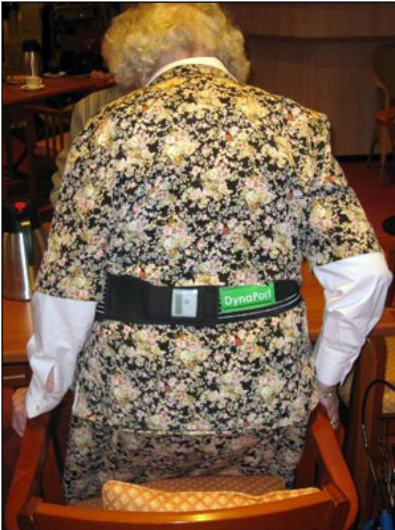
The motion sensors, attached to a belt, can be used to determine if the wearer has fallen.
