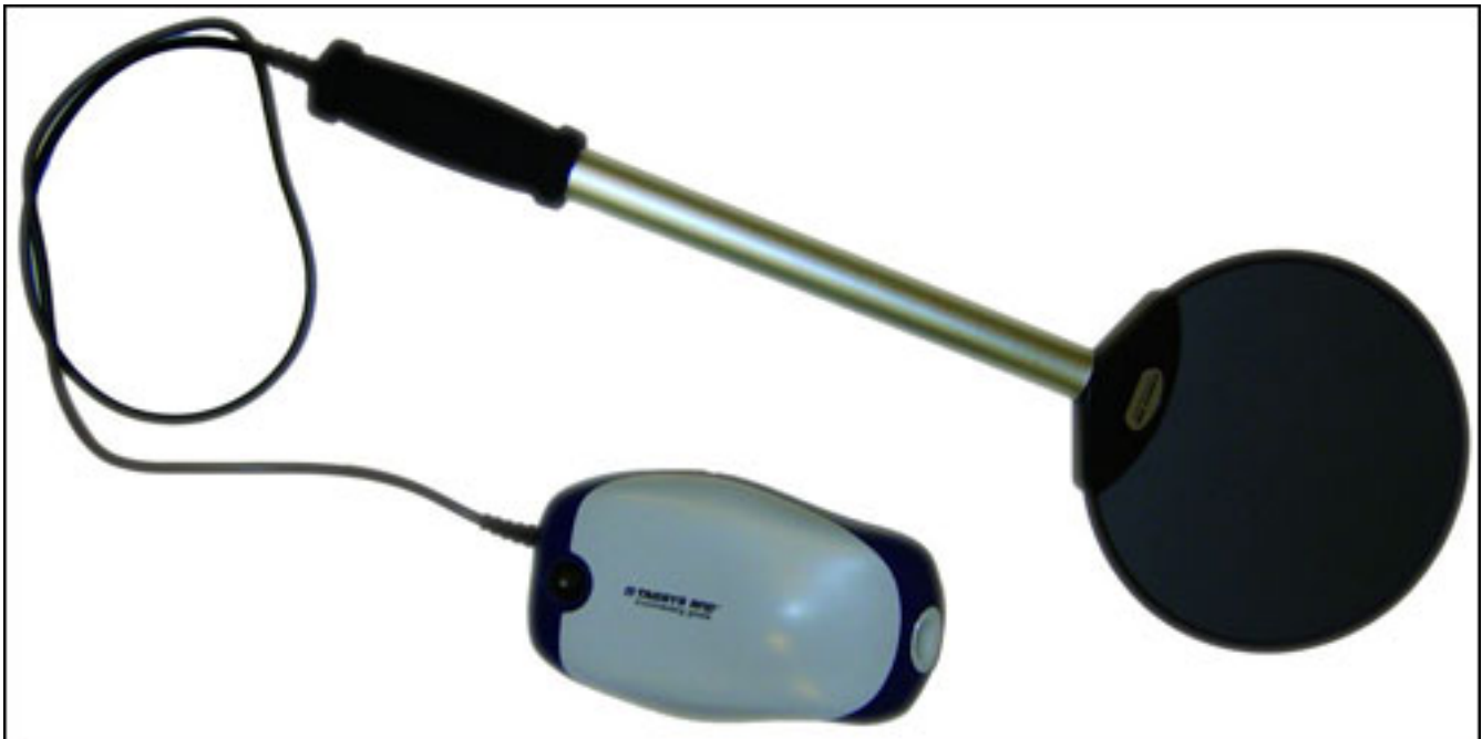
In the store, Rica Lewis salespeople take inventory by means of a mobile Tagsys RFID interrogator and handheld antenna.
