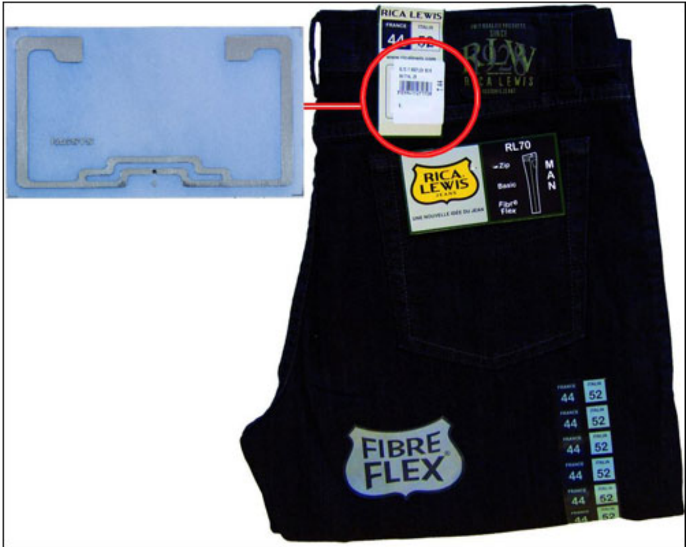
EPC Gen 2 passive tags are embedded in garment labels.
