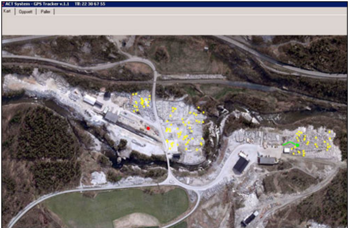
On their onboard computer screen, forklift drivers can view a map indicating where tagged pallets are located, as well as their own position.
