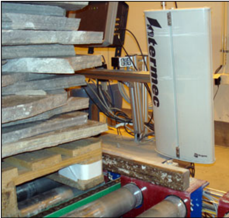
Once an order of finished product is loaded on a pallet and weighed, an Intermec RFID portal reads the ID numbers encoded to the pallet's tags.
