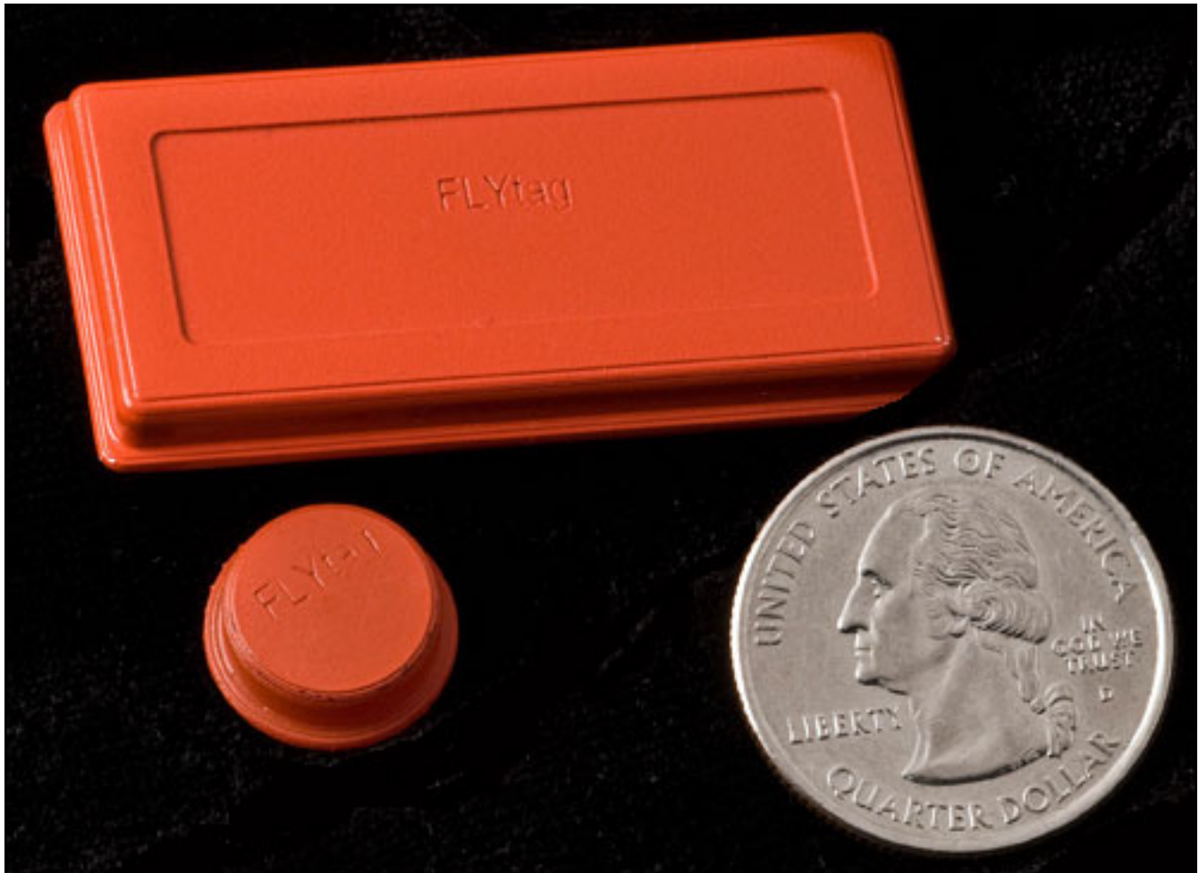
The FLYtag, available in two different sizes, will initially have 4 kilobytes of memory.
