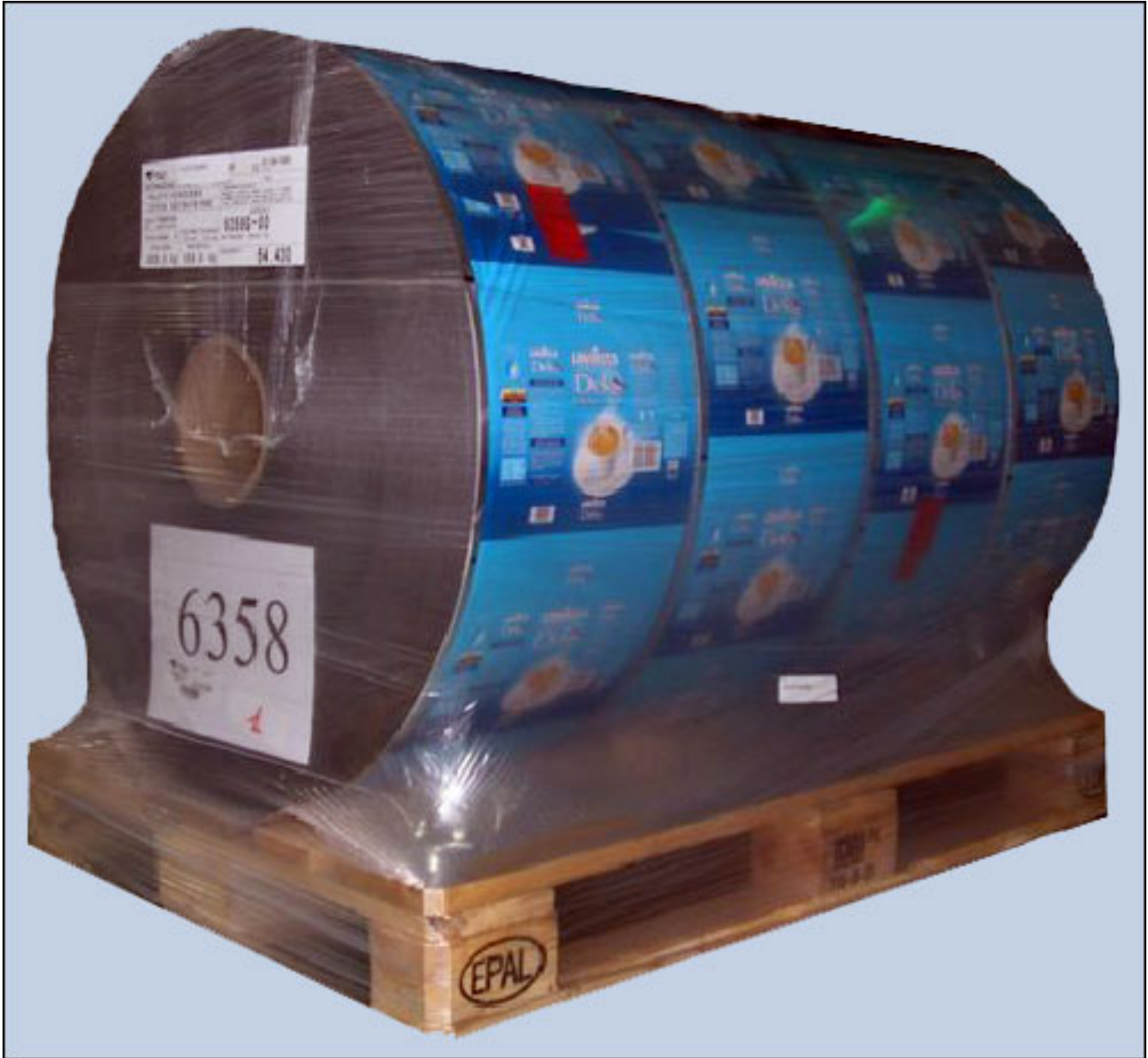
After loading four reels of packaging materials onto a pallet, Goglio Cofibox attaches two adhesive EPC Gen 2 RFID labels onto the exterior of the plastic stretch wrap, as well as an extra tag directly on the pallet.
