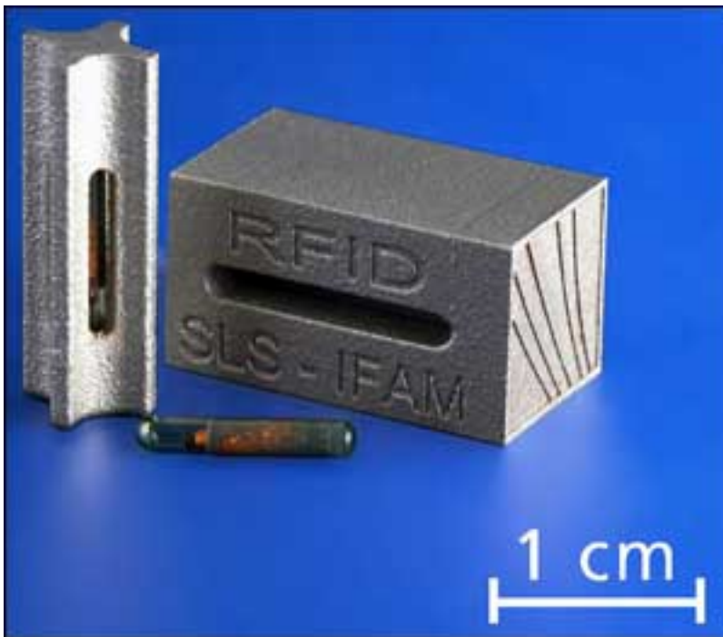
Fraunhofer's researchers used selective laser sintering (SLS) to produce these metallic objects, shown next to a sample of the RFID tag integrated within each item.
