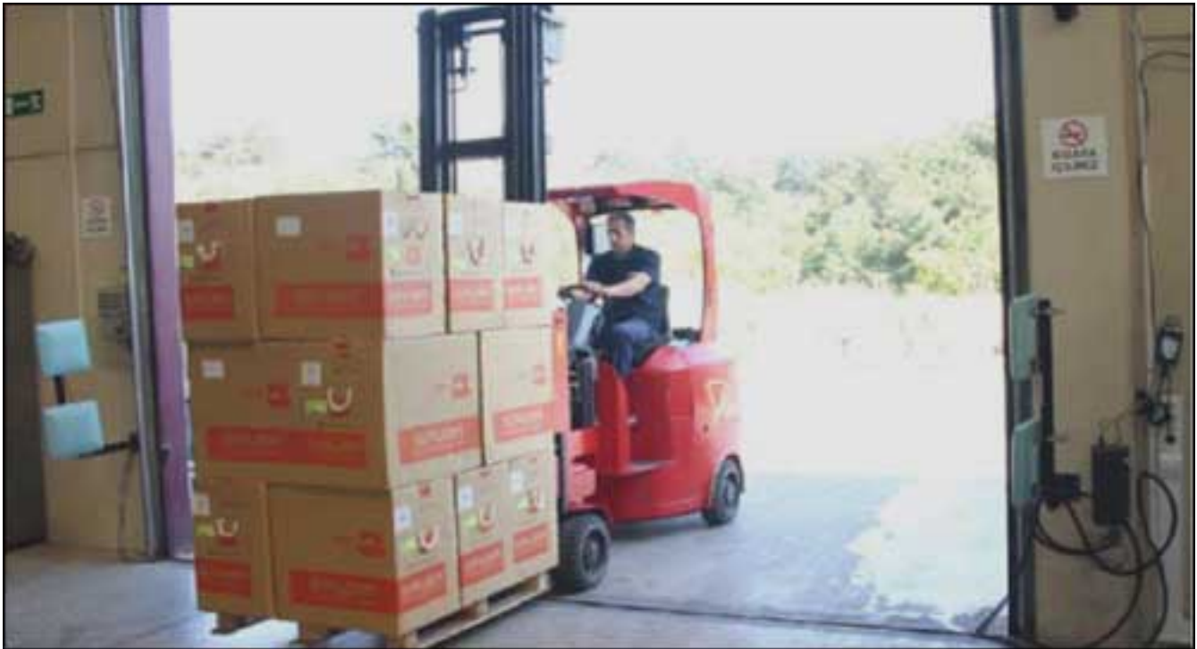
When goods pass through the warehouse entrances and exits, RFID interrogators installed there read the RFID tags on the pallets.
